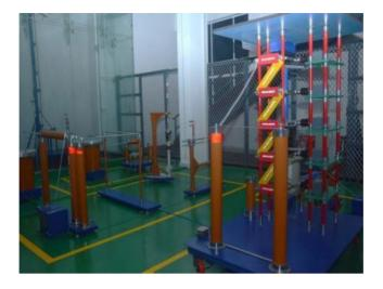
The laboratory is one of few modern High Voltage Laboratories available in the island. High voltage break-down and testing are extensively carried out in the laboratory by the researchers and students Laboratory setups are DC High Voltage Breakdown Tester, High Voltage Tester and Impulse Voltage Generator.
